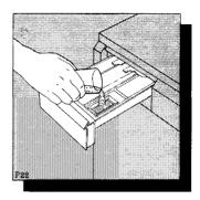
Pour the softener, if required, into the compartment marked **\$**; do not exceed the MAX level.
